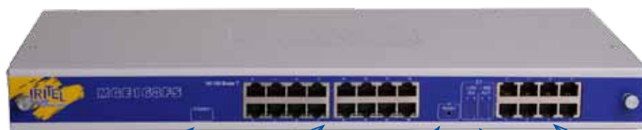
LED napajanje 16 x Fast Ethernet IP reset E1 LED 8 x E1
