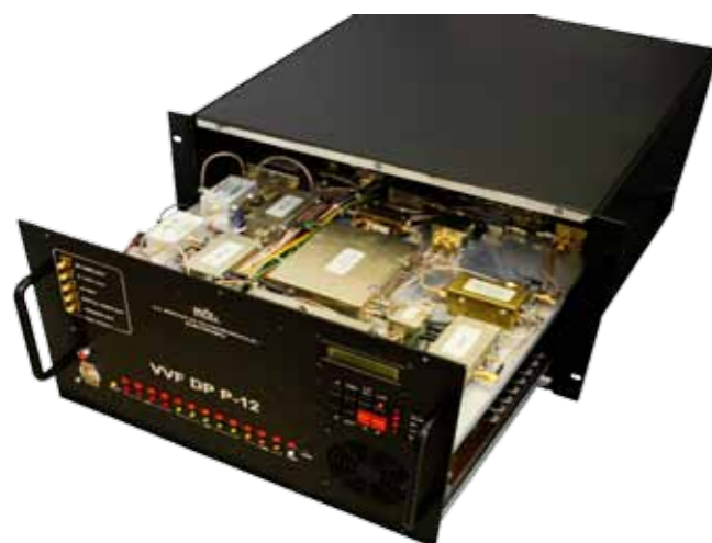
Analog block of receiver
